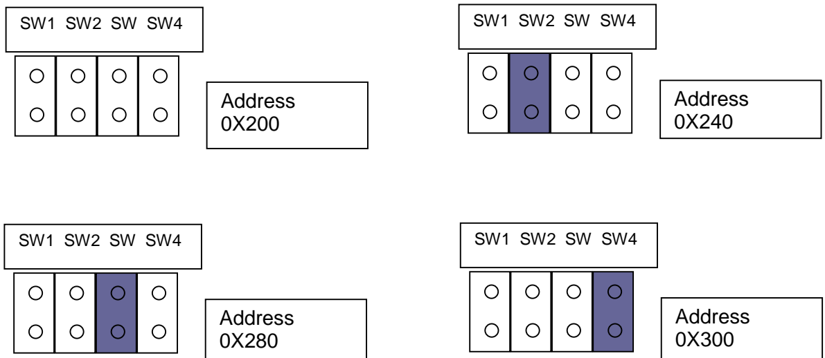
Figure 2-1 Board address selection
